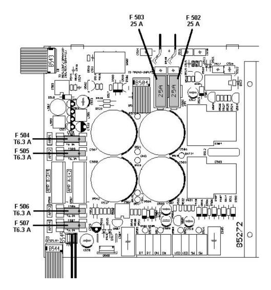
diagram 11 Printed board assembly 85272 showing the position of the DC-fuses F502 to F507
